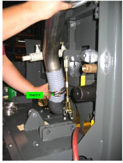
Begin installation of (1) TUBE-SQG SUCTION INTERMEDIATE (3341780) by lubricating outside on short end of the tube and inside of both ends of (1) HOSE-SQUEEGEE TUBE TO GASKET M (3341781). Slide (2) CLAMPS-HOSE 3.5 (3343273) onto flex hose. Slide one end of hose onto short end of tube. Then slide other end of flex hose onto WELD-SQG VAC GASKET MNT 5550.
